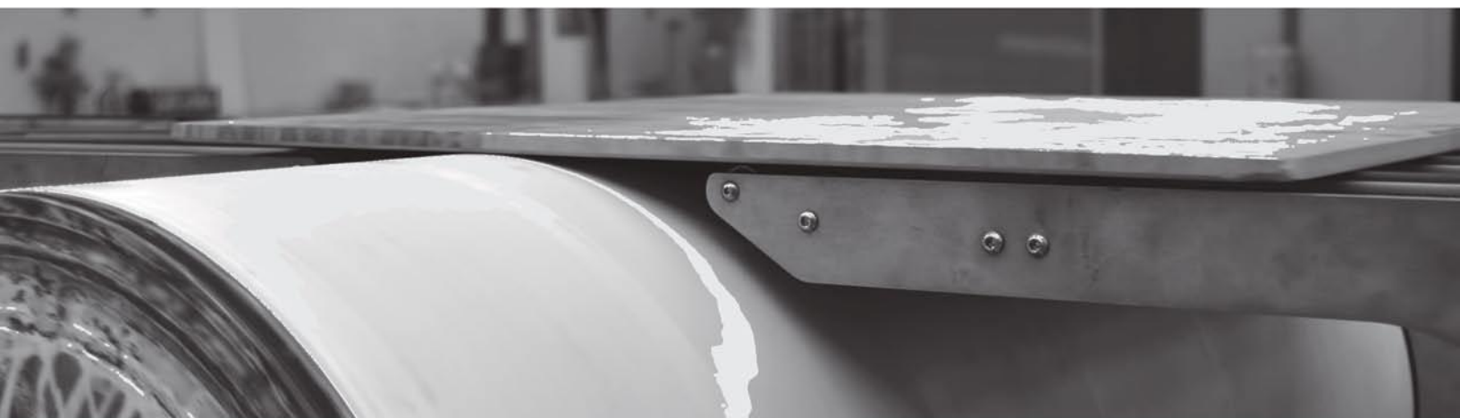
Detail of the problem generated in the kiln ceramic rollers, due to the bad application of the engobe.
