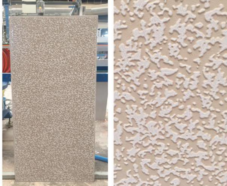
Detail of the application of the slip using BACKPRINT-K, in a 60x120 tile
