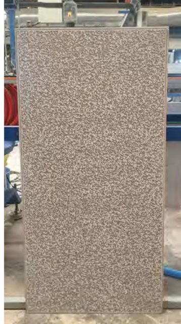
Detail of the application of the engobe using Backprint, in a 60x120 tile.
