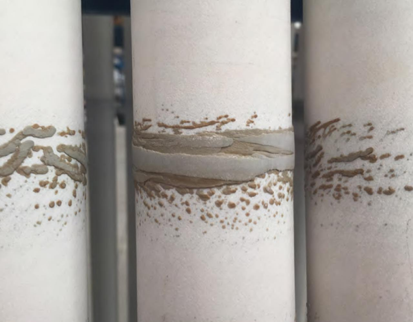
Detail of the problem generated in the kiln ceramic rollers, due to the bad application of the engobe.
