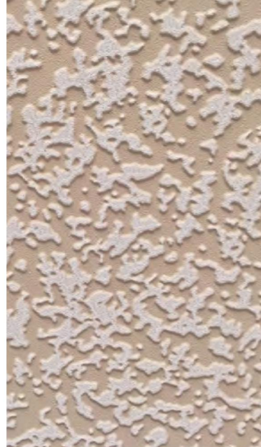
Detail of the application of the engobe using Backprint, in a 60x120 tile.
