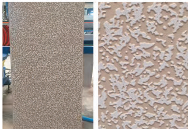
Detail of the engobe application, using BACKPRINT-K Line.
