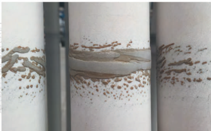
Detail of the problem generated in the kiln ceramic rollers, due to the bad application of the engobe.
